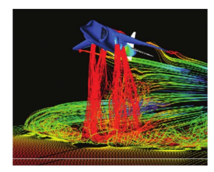
Simulation visualization of the air generated by a Harriet Jet (<u>http://quest.nasa.gov/aero/</u><u>background/tools/</u>)
