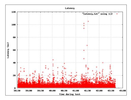
Worst-case latency peaked at just over 100 ms. The way the slow cases are clustered around the same period here is quite common in these results; when the server slows down, it will usually impact all the active clients at that time.
