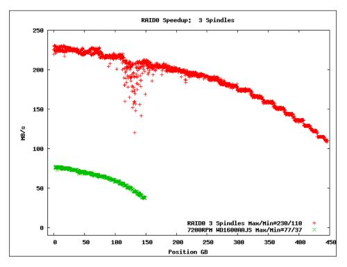
The derived figures from the raw data max and min transfer speed numbers are almost exactly tripled as follows:
