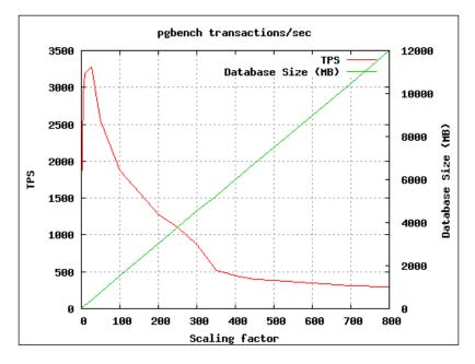
If you look carefully at the left side of this, you can see one of the issues warned about above and in the pgbench documentation: results at a very low database scale are lower than when the database is a bit larger. This is due to lock contention for the small branches table in particular, when running at higher client counts with a tiny scale.
