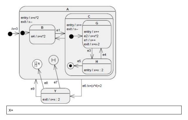
(open box) E - You are given the following state machine diagram. What is the value of x after the occurrence of the event chain: e1 e3 e5 e2?
