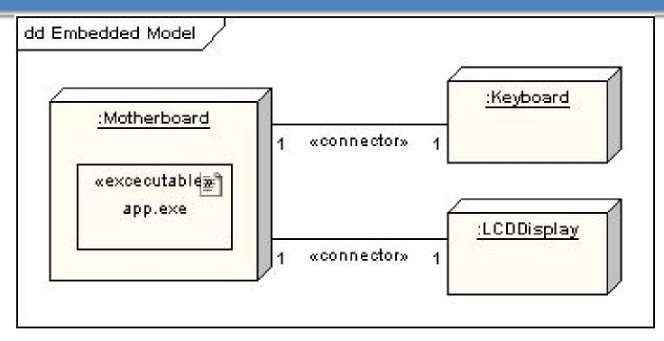
Deployment diagrams to part of the embedded system, presenting an executable artifact as being contained by the motherboard node
