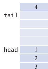
Figure 16 A Queue That Wraps Around the End of the Array
