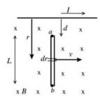
The magnetic field of the wire is given by  $B = \frac{\mu_0 I}{2\pi r}$  and varies along the length of the bar. At every point along the bar  $\vec{B}$  has direction into the page.
