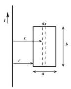
Consider a narrow strip of width dx and a distance x from the long wire, as shown in Figure 29.53a. The magnetic field of the wire at the strip is  $B = \mu_0 I/2\pi x$ . The flux through the strip is  $d\Phi_B = Bb \ dx = (\mu_0 Ib/2\pi)(dx/x)$ .
