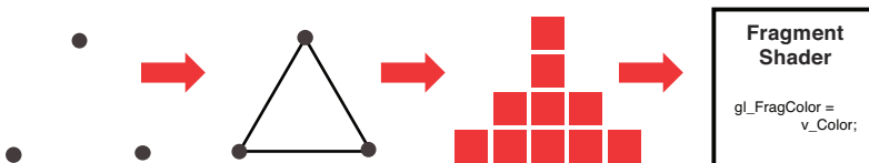
Figure 5.9 Vertex coordinate, identification of a triangle from the vertex coordinates, rasterization, and execution of a fragment shader
