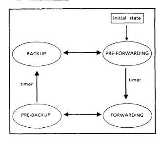
Upon startup, bridge B initializes each link to be in the PRE\_FORWARDING state, with the link database for each link initialized to claim B as the Root, B as the Designated Bridge on that link, B's distance from the Root to be 0, and the timer set to PRE\_FORWARDING\_DELAY.
