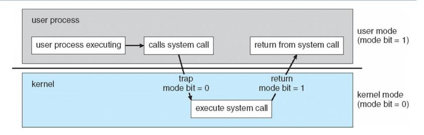
**Dual-mode** operation allows OS to protect itself and other system components
