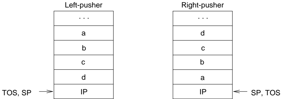
Figure 13.2 Two ways of pushing parameters onto the stack.
