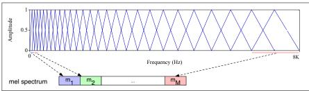
Figure 26.5 The mel filter bank (Davis and Mermelstein, 1980). Each triangular filter, spaced logarithmically along the mel scale, collects energy from a given frequency range.
