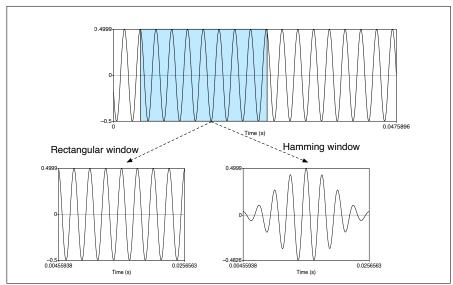
Windowing a sine wave with the rectangular or Hamming windows. **Figure 26.3**
