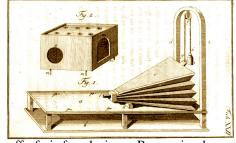
small auxiliary bellows to provide the puff of air for plosives. By moving levers with both hands to open and close apertures, and adjusting the flexible leather "vocal tract", an operator could produce different consonants and vowels.
