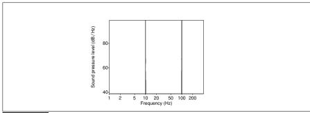
Figure 25.16 The spectrum of the waveform in Fig. 25.15.
