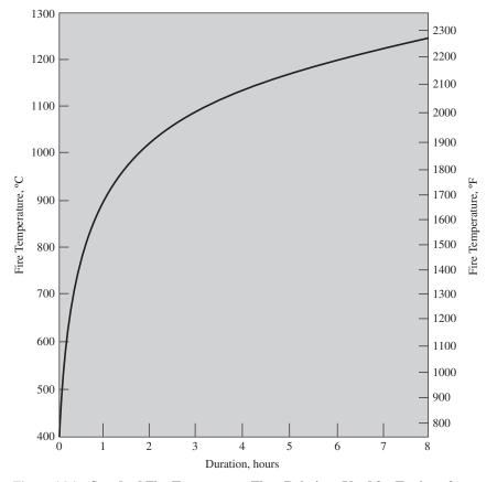
Figure 16.1 Standard Fire Temperature-Time Relations Used for Testing of **Building Elements**
