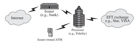
(a) Point-to-point connection to processor
