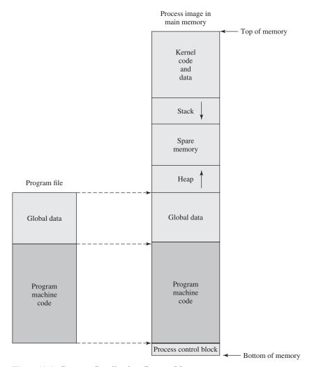
Figure 10.4 Program Loading into Process Memory
