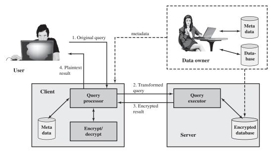
Figure 5.9 A Database Encryption Scheme
