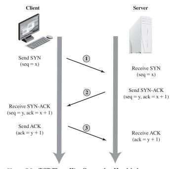
Figure 7.2 TCP Three-Way Connection Handshake
