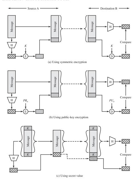
Figure 2.5 Message Authentication Using a One-Way Hash Function
