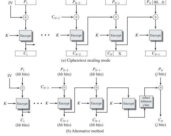
Figure 20.12 Block Cipher Modes for Plaintext Not a Multiple of Block Size
