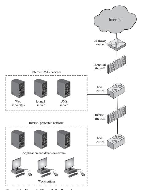
Figure 9.2 Example Firewall Configuration
