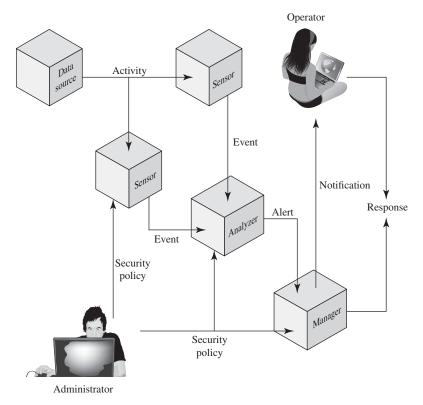
Figure 8.7 Model for Intrusion Detection Message Exchange
