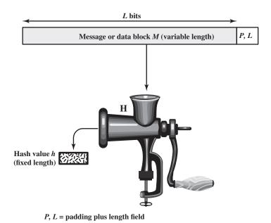
Figure 2.4 Cryptographic Hash Function; h = H(M)
