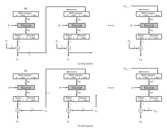
Figure 20.7 s-bit Cipher Feedback (CFB) Mode
