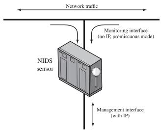
Figure 8.4 Passive NIDS Sensor Source: Based on [CREM06].
