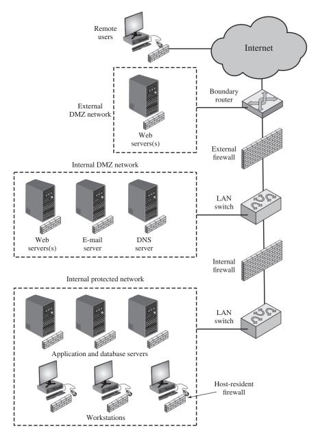
Figure 9.4 Example Distributed Firewall Configuration
