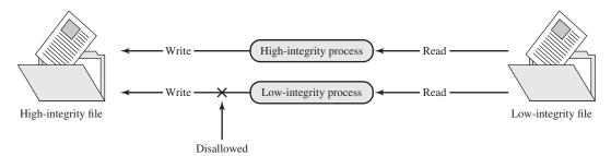
Figure 13.4 Contamination with Simple Integrity Controls Source: [GASS88].
