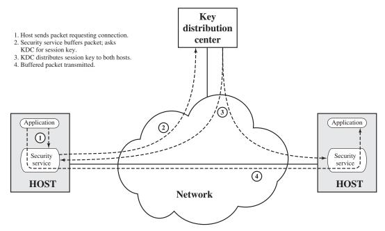
**Figure 20.10 Automatic Key Distribution for Connection-Oriented Protocd**
