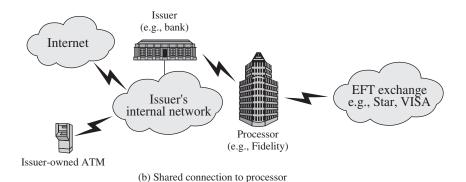
Figure 3.14 ATM Architectures Most small to mid-sized issuers of debit cards contract processors to provide core data processing and electronic funds transfer (EFT) services. The bank's ATM machine may link directly to the processor or to the bank.
