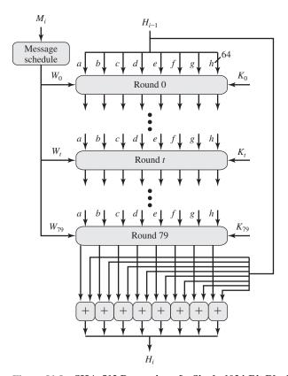
Figure 21.3 SHA-512 Processing of a Single 1024-Bit Block
