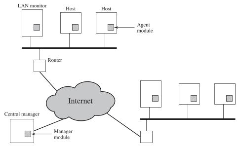
Figure 8.2 Architecture for Distributed Intrusion Detection
