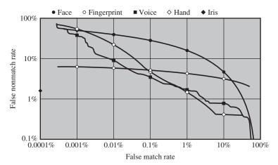
Figure 3.11 Actual Biometric Measurement Operating Characteristic **Curves, Reported in [MANSO1]** To clarify differences among systems, a log-log scale is used.
