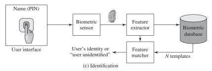
**Figure 3.8 A Generic Biometric System** Enrollment creates an association between a user and the user's biometric characteristics. Depending on the application, user authentication either involves verifying that a claimed user is the actual user or identifying an unknown user.
