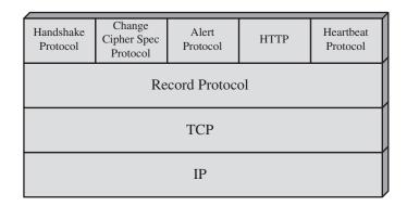
Figure 22.4 SSL/TLS Protocol Stack
