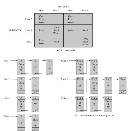
Figure 4.2 Example of Access Control Structures
