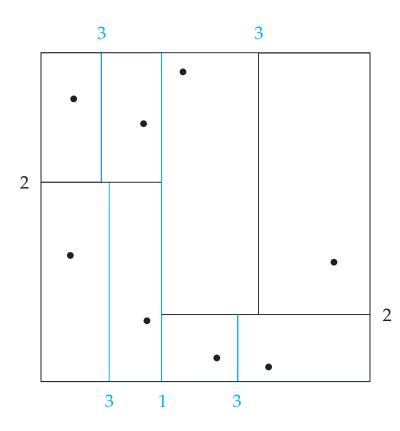
The k-d-B tree extends the k-d tree to allow multiple child nodes for each internal node; well-suited for secondary storage.
